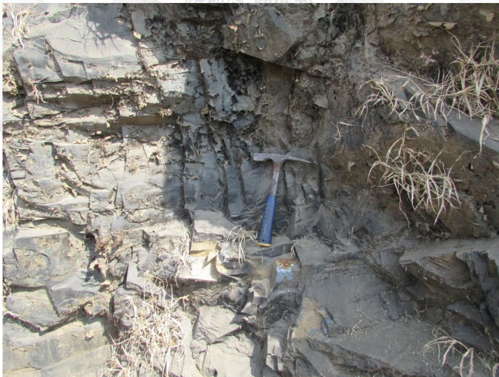
Fig. 1.4: Argillite exposed near Anjuna Dam along Chorla Ghat section.
