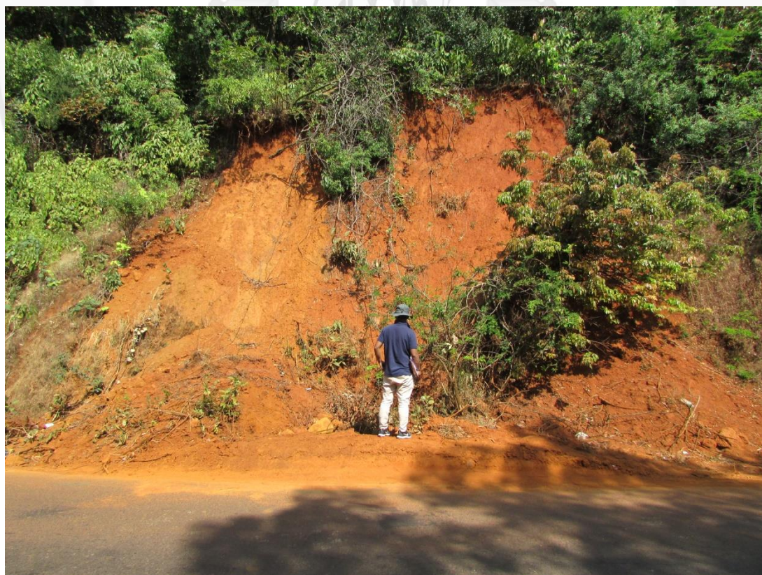
Fig. 4.24: Regolith Thickness 0.5 - 5\text{ m} near Chorla along Chorla Ghat section.
