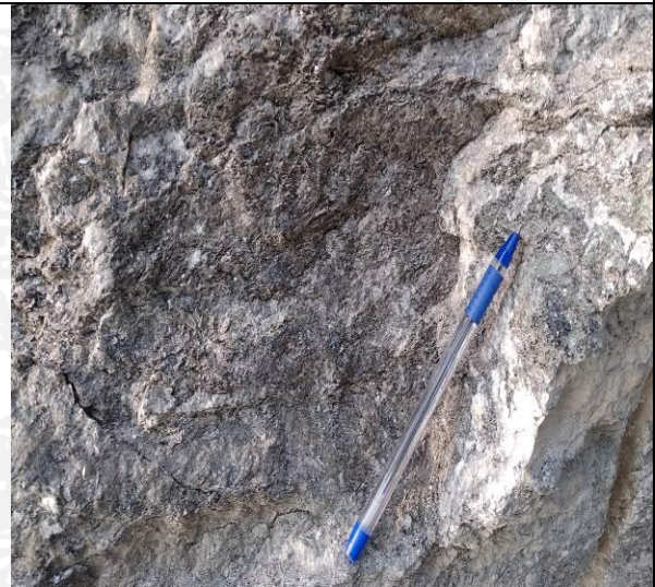
Fig. 2.1d Micaceous minerals developed along the weak planes of granite gneiss
